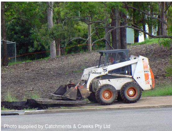
Photo 11 – Skid-steer loader (“bobcat” is a commercial brand name)
