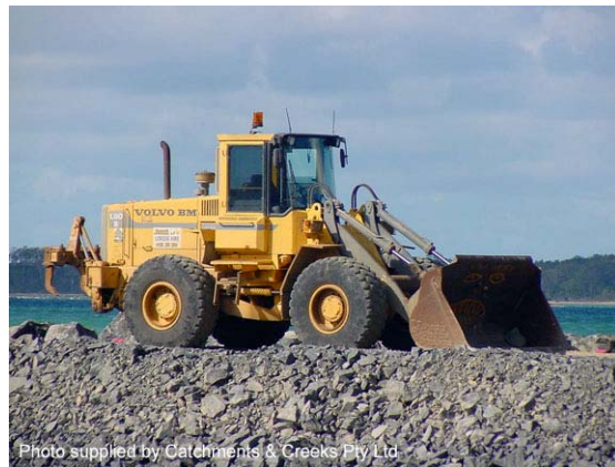
Photo 8 – Loader (wheel loader), crawler loaders are also available
