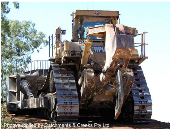
Photo 3 – Crawler dozer with ripper (rear attachment)
