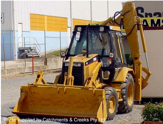
Photo 1 – Backhoe/loader, the “hoe” being attached to the rear of the unit, hence the name ‘backhoe’
