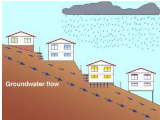
Normal groundwater flow down a slope
