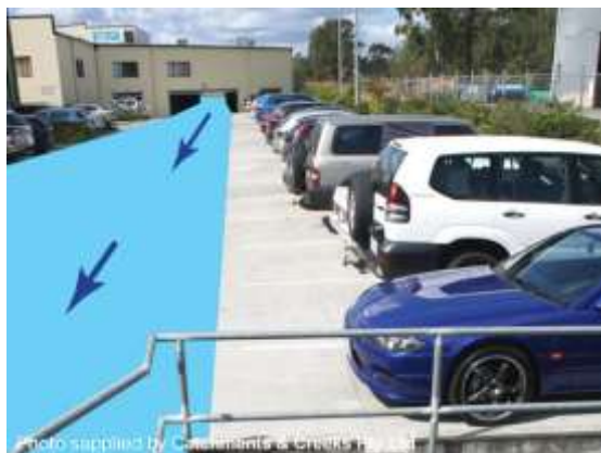
Overland flow path passing under building
