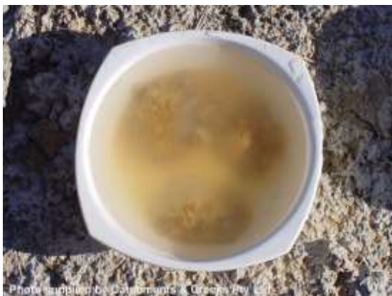
Field testing a dispersive soil
