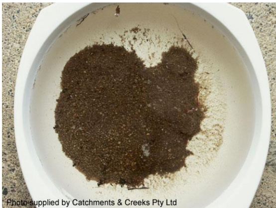
Collapse of a slaking soil in water
