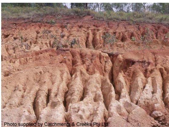
Fluting erosion in a dispersive soil
