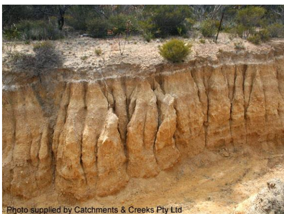
Fluting erosion in a dispersive soil
