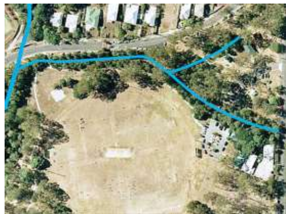
Aerial image showing channel alignment
