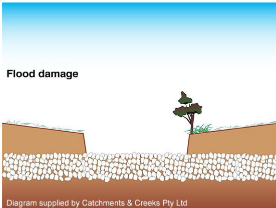
Enlarged, post-flood channel
