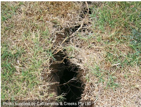
Crack several metres from a creek bank
