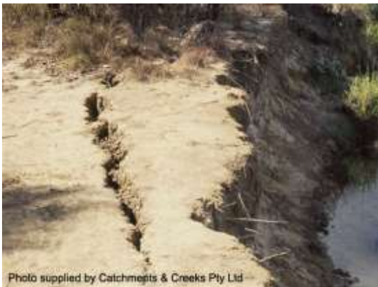
Cracks along the edge of the bank (Qld)
