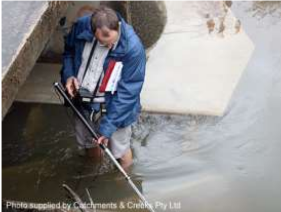
Measuring local flow velocity at a culvert
