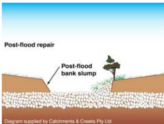
Possible post-flood creek rehabilitation
