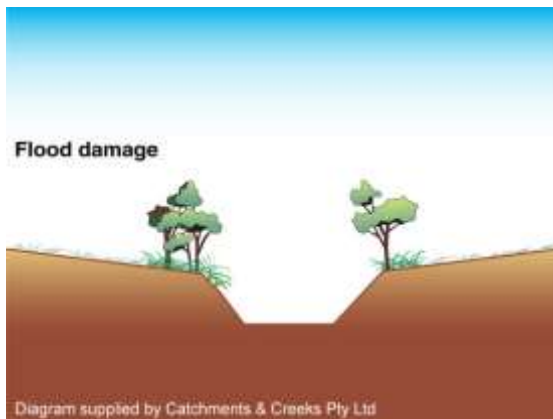
Enlarged, post-flood channel
