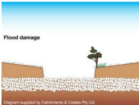
Enlarged, post-flood channel
