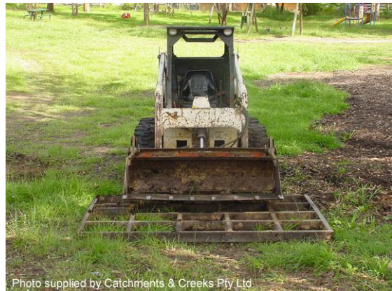
Skid-steer topsoil leveller/spreader
