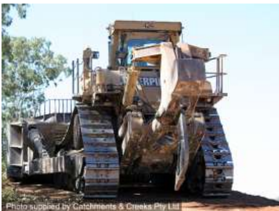
Deep ripper (for ripping hard soil)
