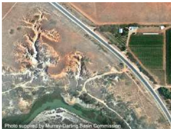
Branching of gully erosion (SA)
