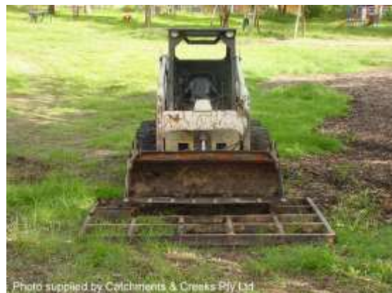
Skid-steer topsoil leveller/spreader
