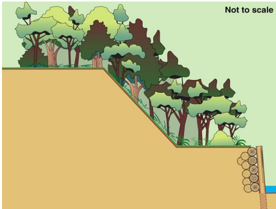
Brushwood toe protection
