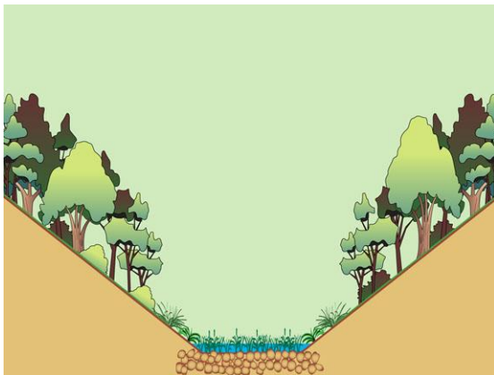
Straight channel with steep bed slope
