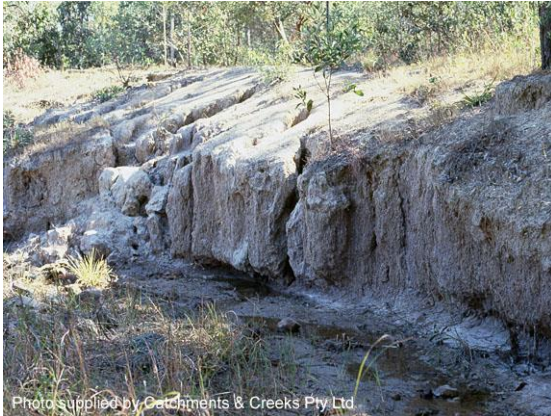
Dispersive soil erosion near the main bank
