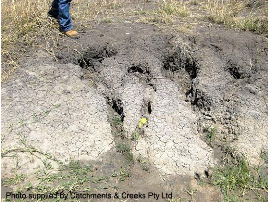
Deep rilling and outlet of tunnels (Qld)
