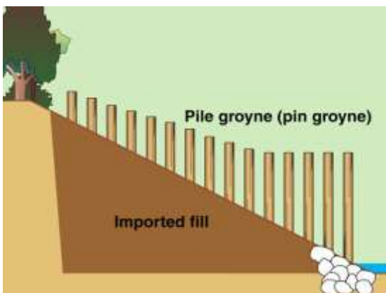
Pile field bank stabilisation
