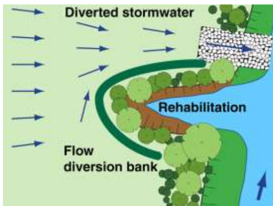
Divert stormwater away from the gully
