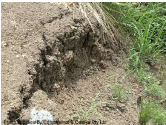
Dry, cracking clay (Qld)
