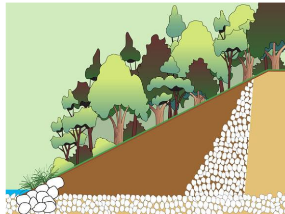
Stage 3: Bank revegetation
