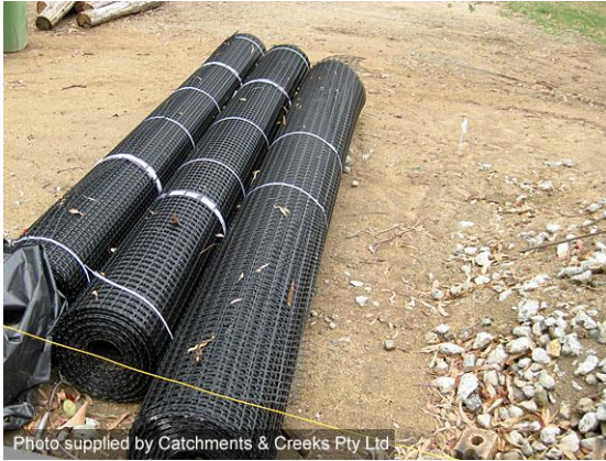
Earth reinforcing mesh (Qld)
