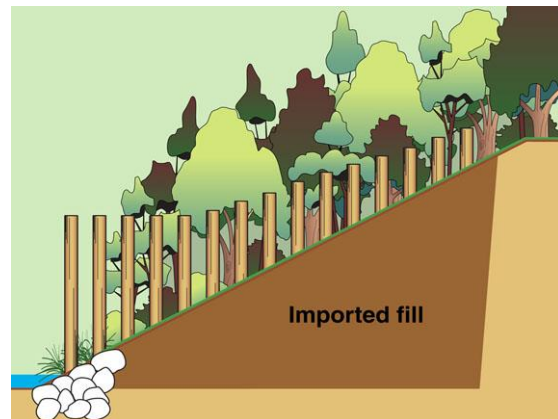
Stage 3: Bank revegetation
