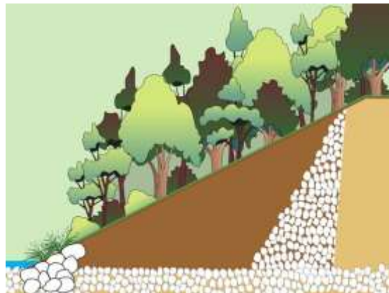
Stage 3: Bank revegetation
