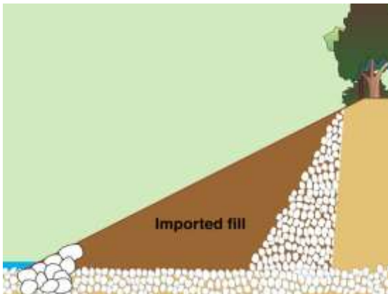
Stage 2: Cover gravel with imported fill
