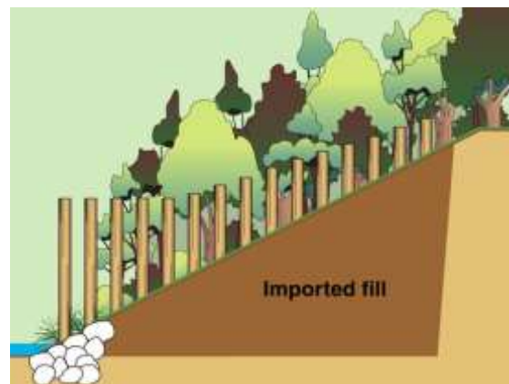
Stage 3: Bank revegetation
