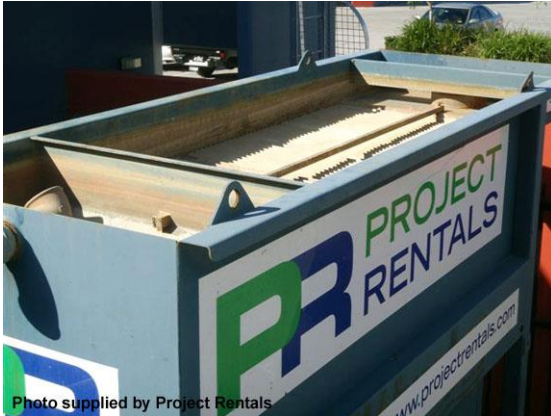
Lamella settling tank
