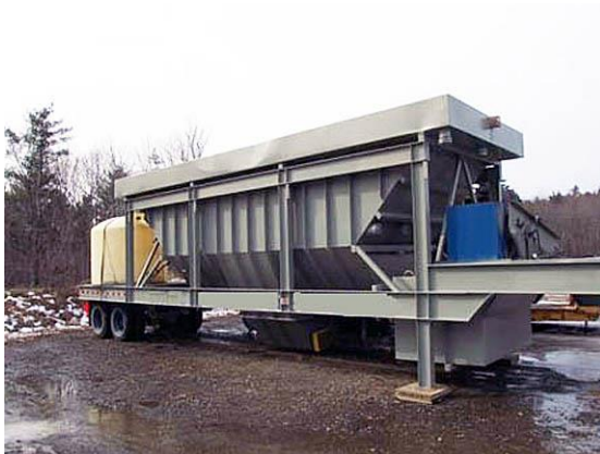
Mobile clarifier tank
