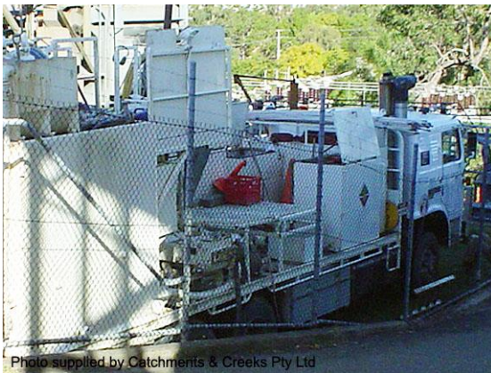
Truck-mounted centrifuge (Qld)
