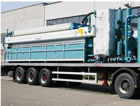
Truck-mounted filter press
