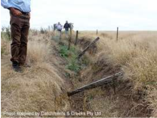
Photo supplied by Catchments & Creeks Pty Ltd Inspection of gully erosion (Qld)
