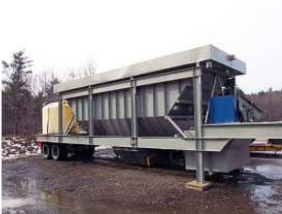
Mobile clarifier tank
