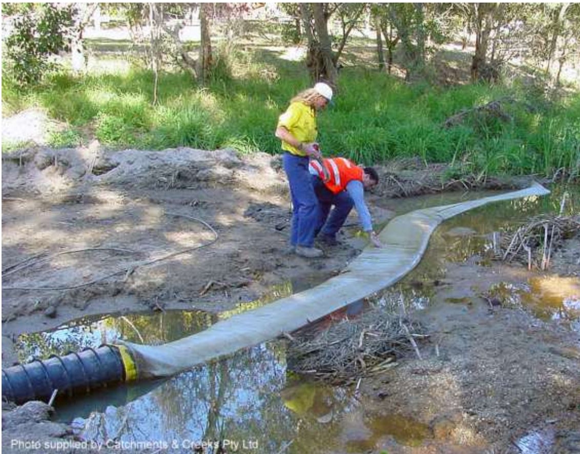
Initial testing of the filter tube concept in Brisbane
