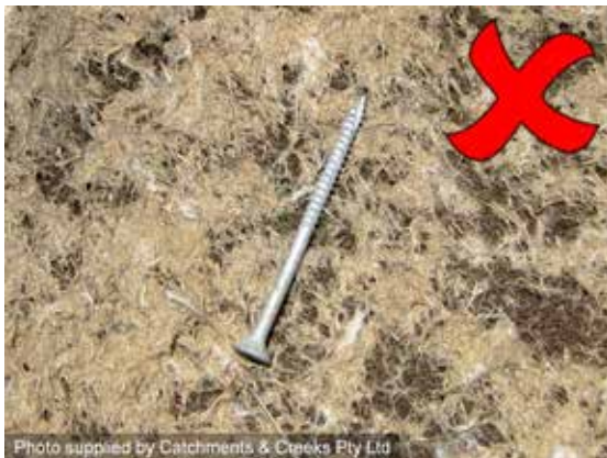
Wood screws used to anchor a blanket
