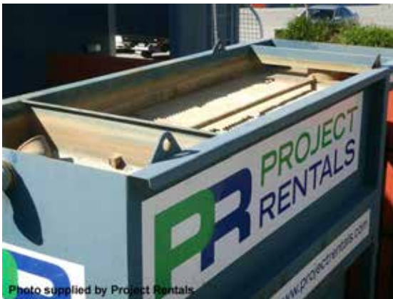
Lamella settling tank
