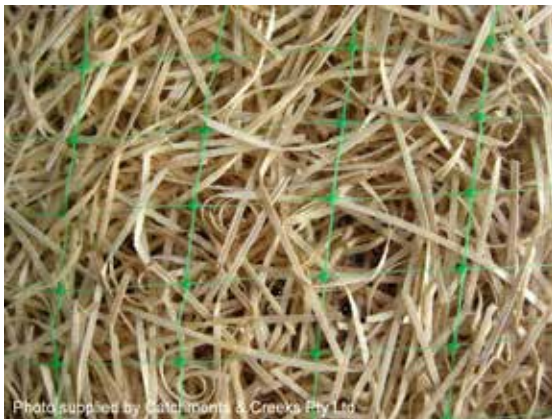
Temporary erosion control mat
