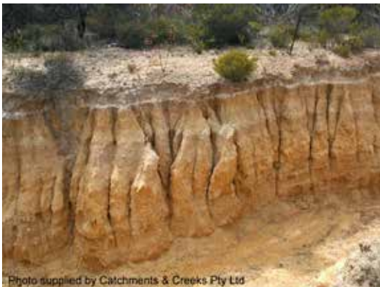
'Fluting' erosion within a dispersive soil
