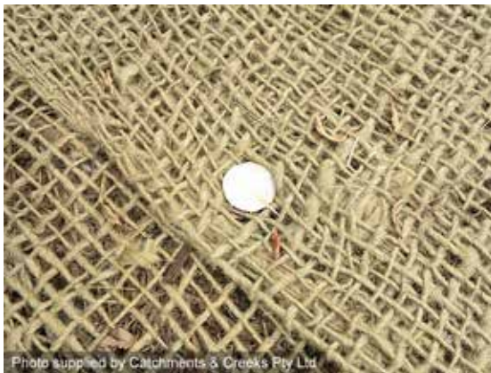
Erosion control mesh
