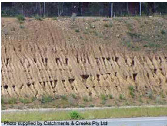
A form of rilling known as 'fluting'
