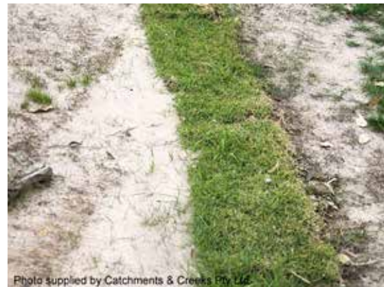
Grass filter strip with captured sediment
