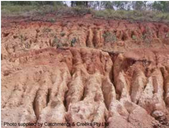
'Fluting' erosion within a dispersive soil
