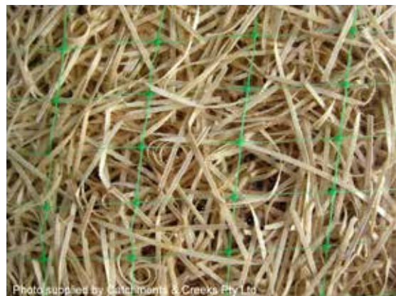
Non UV-stabilised synthetic composite mat
