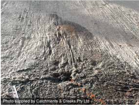
Spring water visible on jute blanket
