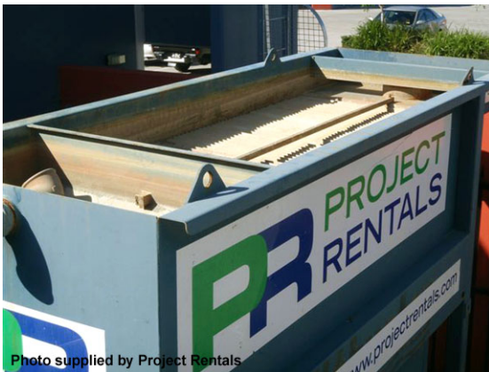
Lamella settling tank
