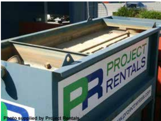
Lamella settling tank
