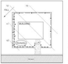
**Erosion & Sediment Control Plan**
