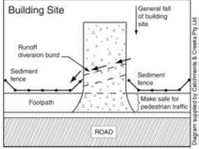
Rock pad with flow diversion berm
