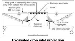
Excavated drop inlet protection
