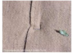
Temporary (jute) erosion control blanket
