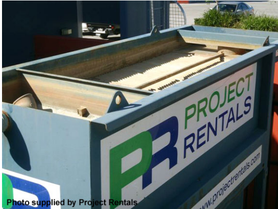
Lamella settling tank
