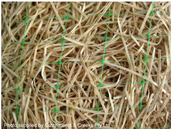
Temporary erosion control mat
