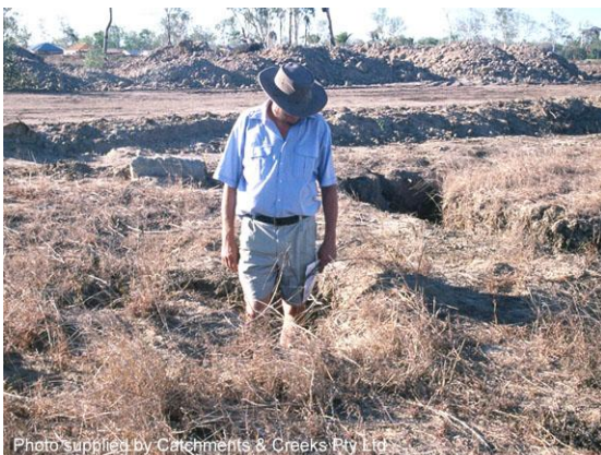
Severe tunnelling within a dispersive soil
