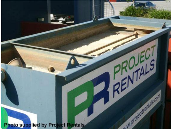
Portable settling (lamella) tank
