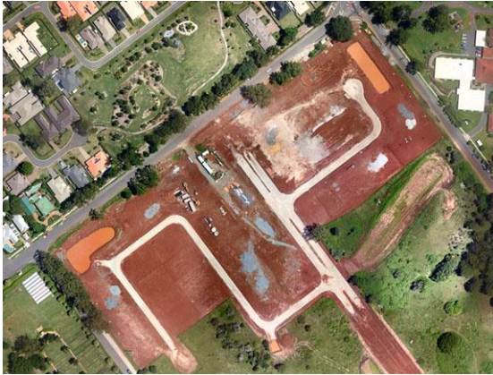
Construction site with sediment basins
