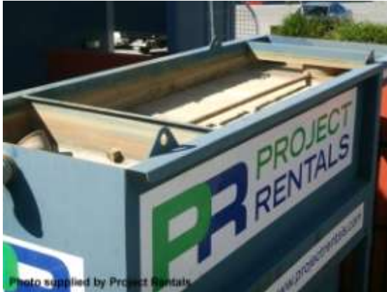
Portable settling (lamella) tank
