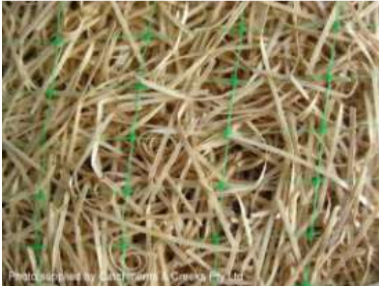
Temporary erosion control mat
