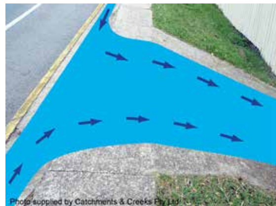
Water spilling down modified driveway
