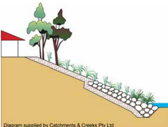
Bank stabilisation works
