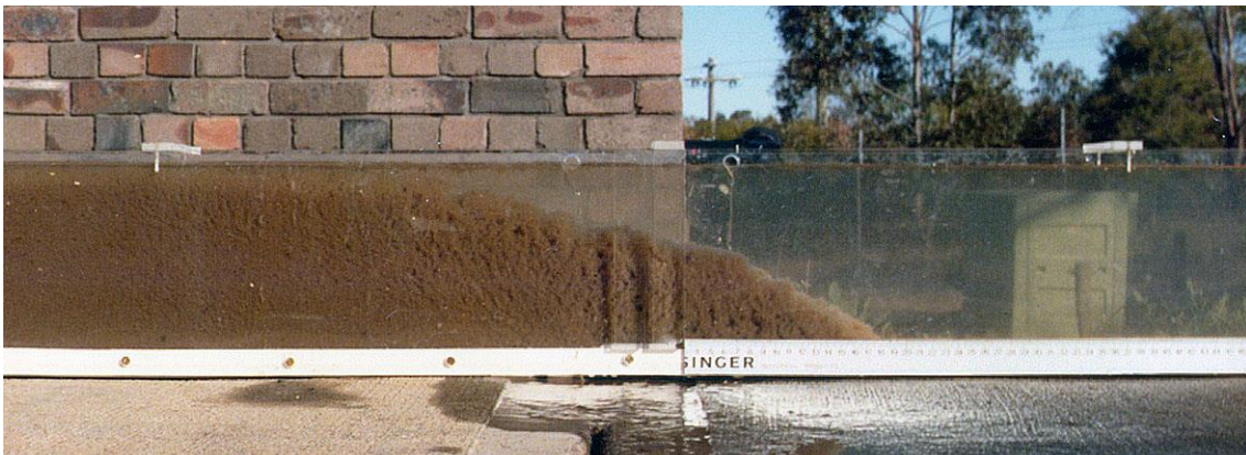
Lock exchange tank used to measure density difference of wastewater floc (NSW)
