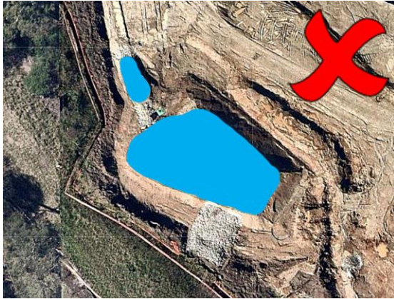
Inadequate forebay width
