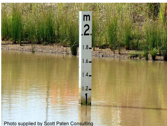
Sediment storage depth marker (Qld)
