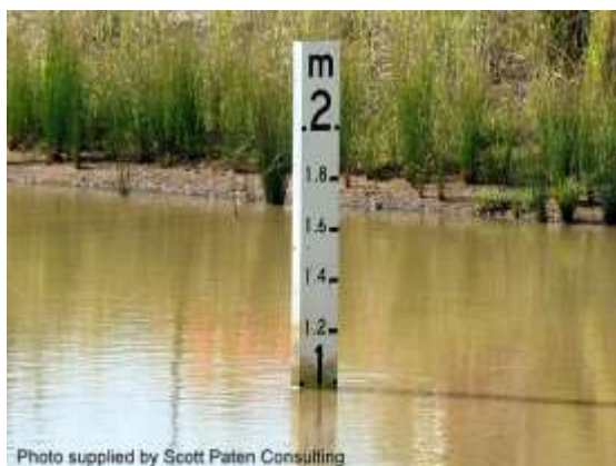
Sediment storage depth marker (Qld)
