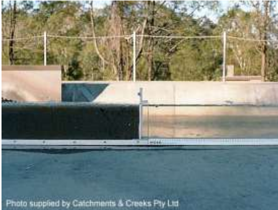
Loch exchange test prior to gate removal
