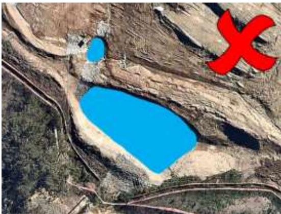
Forebay not aligned with basin
