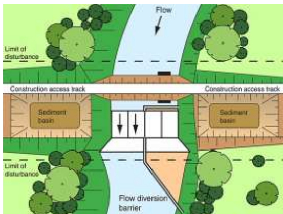
Basins located within a road reserve
