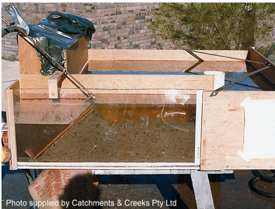
Sludge scour test unit, 1986
