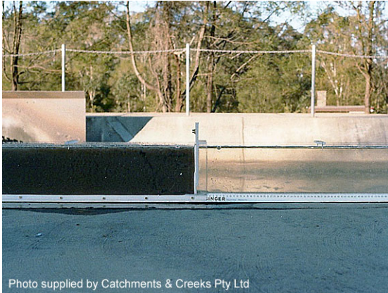
Lock exchange test prior to gate removal
