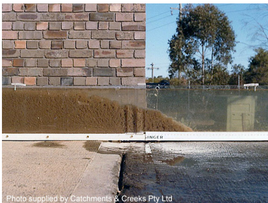
Lock exchange test after gate removal
