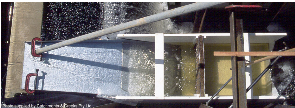
Weir flow measurement using a triangular-notch, thin-plate weir (1986)
