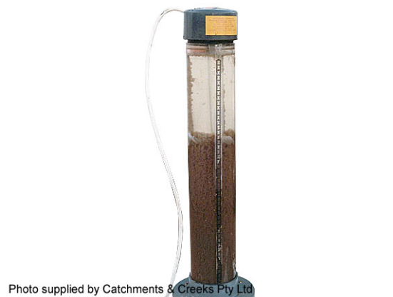
Stirred sludge volume index (SSVI) test
