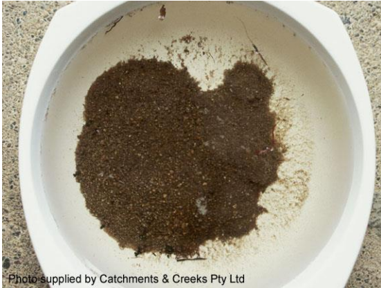
Collapse of a slaking soil in water
