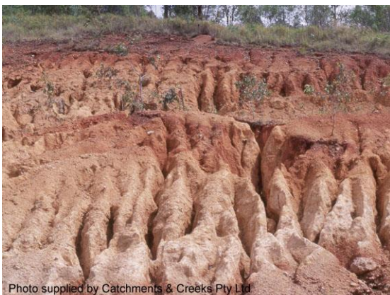
Fluting erosion in a dispersive soil (Qld)
