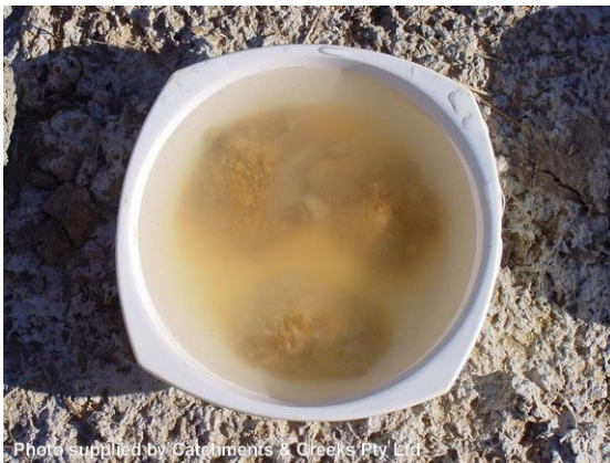
Dispersion of a dispersive soil
