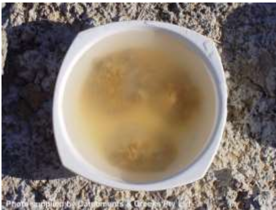
Dispersion of a dispersive soil
