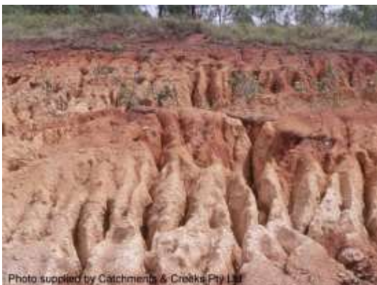
Fluting erosion in a dispersive soil (Qld)
