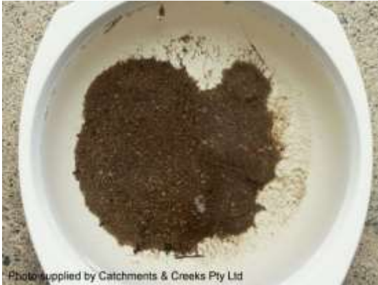
Collapse of a slaking soil in water
