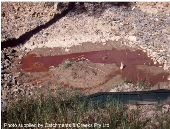
Runoff from an exposed acid sulfate soil
