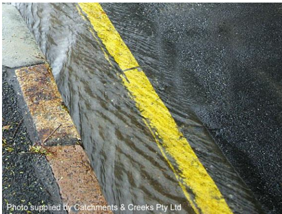
Shock lines on supercritical flow
