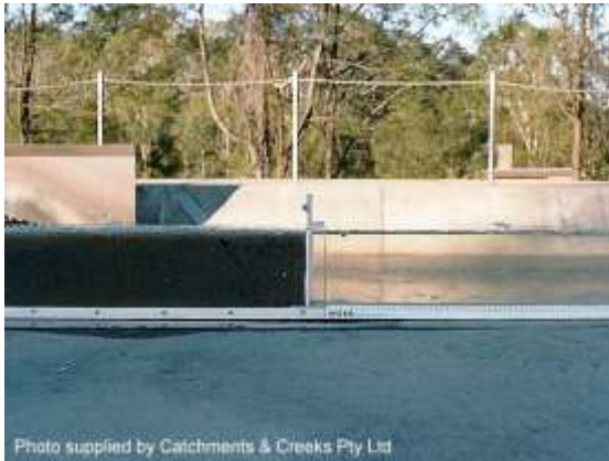
Lock exchange test prior to gate removal
