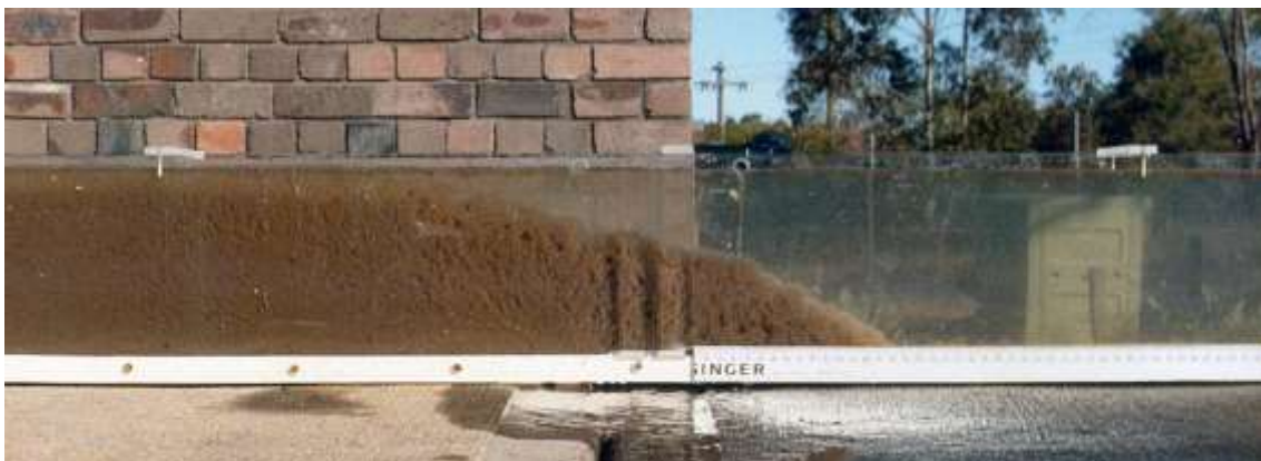
Lock exchange tank used to measure density difference of wastewater floc
