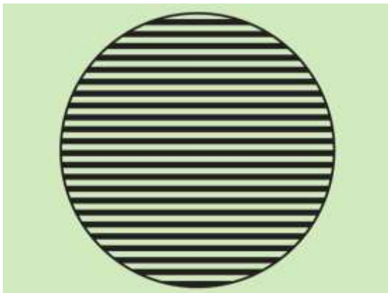
Horizontally aligned filter (50%)
