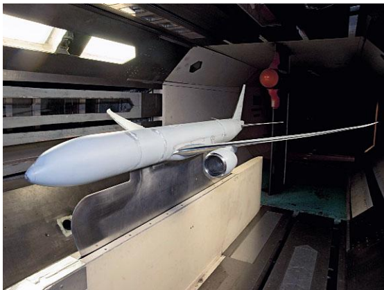
Wind tunnel testing of a Boeing 777
