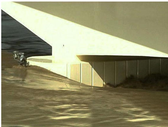
Subcritical flow around a bridge pier
