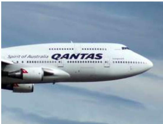
The rounded nose of a subsonic jet
