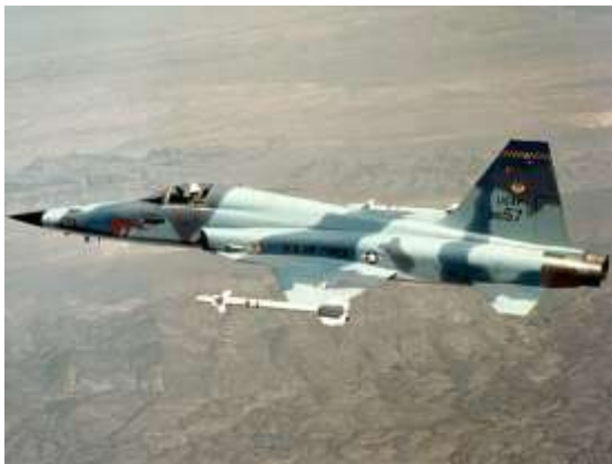
Note long engine intake tunnel
