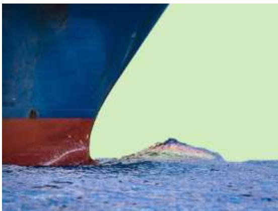
Supercritical flow with a bulbous bow
