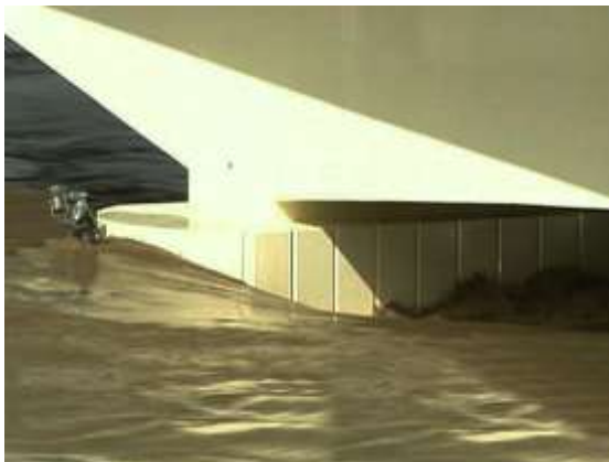
Subcritical flow around a bridge pier
