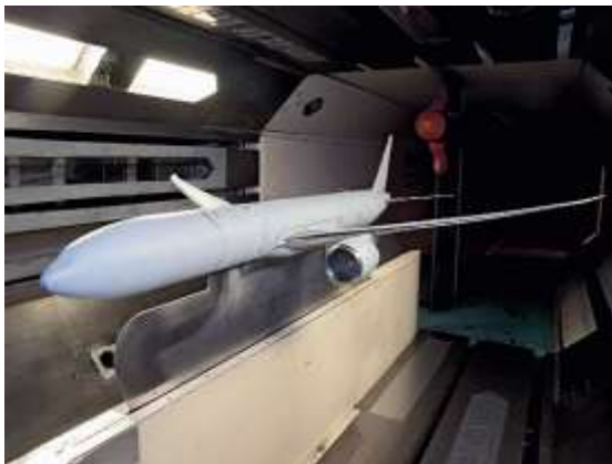
Wind tunnel testing of a Boeing 777
