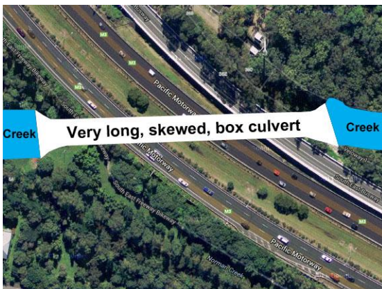
Long culvert under a motorway
