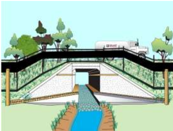
Single cell culvert with low-flow channel
