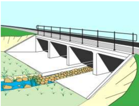
Multi-cell culvert with a low-flow channel
