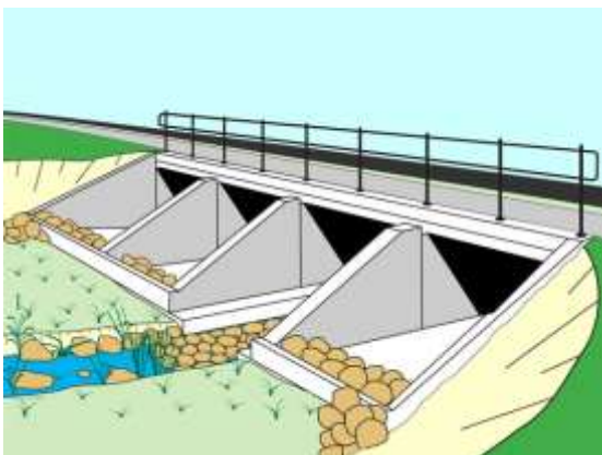
Culvert with a recessed wet cell
