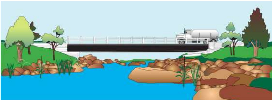
Single span steel girder bridge
