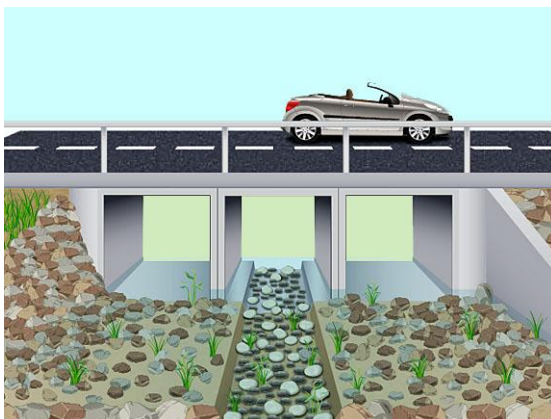
Fish-friendly, multi-cell box culvert
