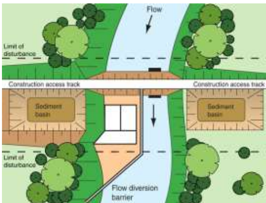
Staged culvert construction (ESCP)
