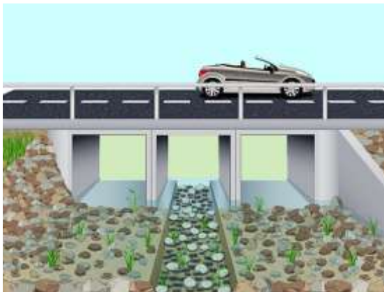
Fish-friendly, multi-cell box culvert
