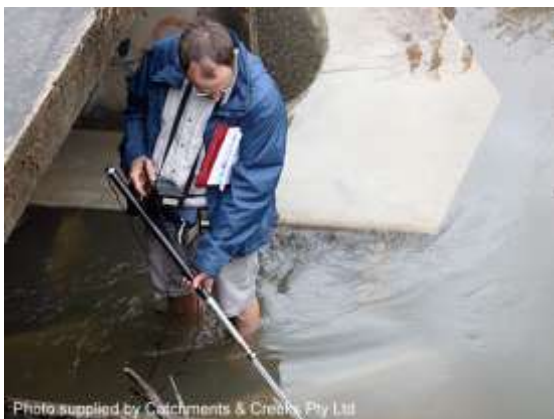
Measuring local flow velocity (Qld)
