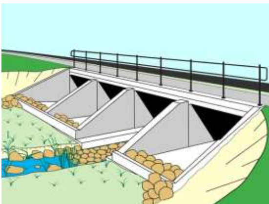
Culvert with low-flow cell
