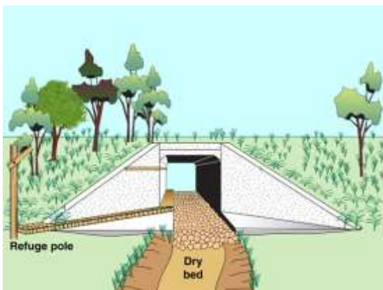
Single cell culvert on an ephemeral creek
