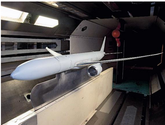
Wind tunnel testing of a Boeing 777
