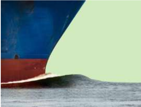
Subcritical flow with a bulbous bow
