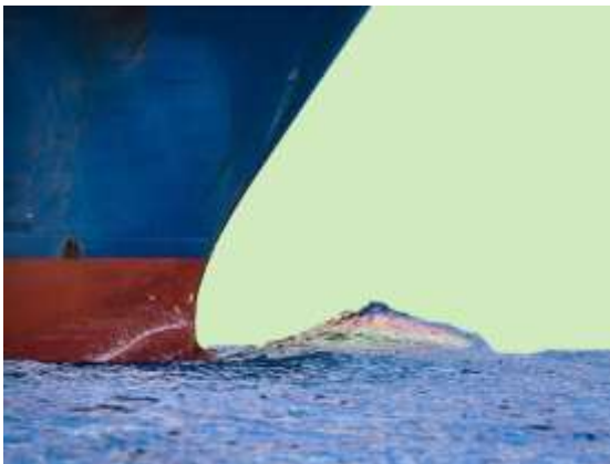
Submerged bulbous bow
