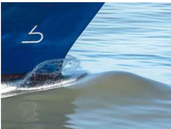
Well submerged bulbous bow
