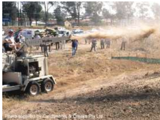
Straw mulcher with bitumen spray
