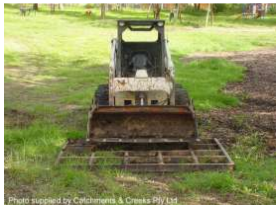
Skid-steer topsoil leveller/spreader
