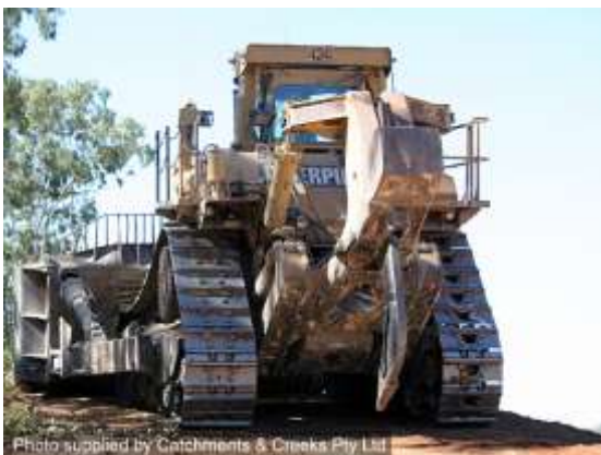
Deep ripper (for ripping hard soil)
