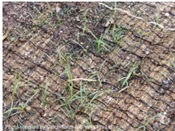
Erosion control mat (composite material)
