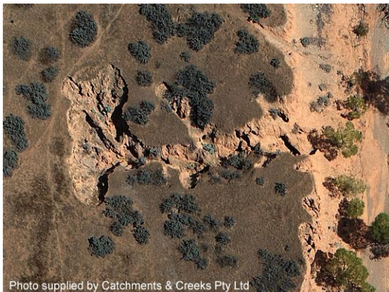
Lateral bank erosion (SA)
