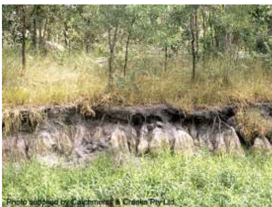
Exposure of a dispersive subsoil (Qld)
