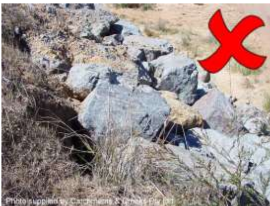
Erosion under rocks on a dispersive soil
