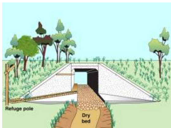
Single cell culvert on an ephemeral creek
