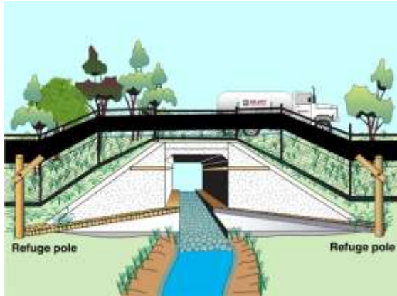
Fauna culvert with exclusion fencing
