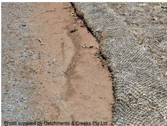
Crushed fibre roll
