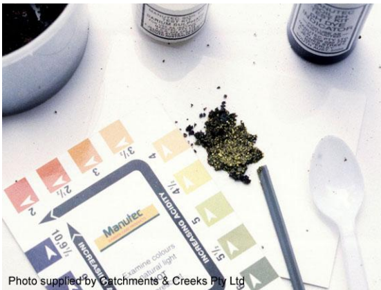
Field testing of soil pH
