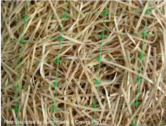
Temporary erosion control mat
