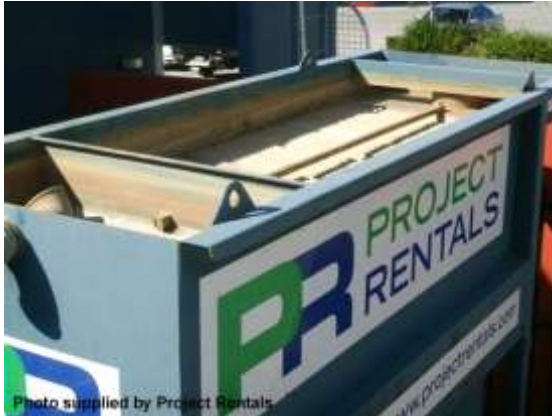
Portable settling (Lamella) tank
