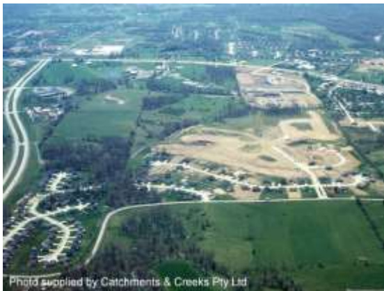
Staged land clearing
