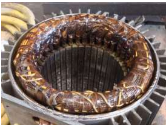
Burnt wiring of an electric motor
