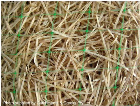
Temporary erosion control mat
