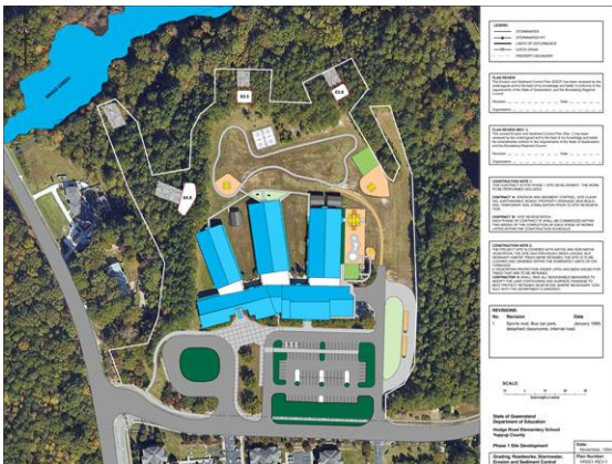
Revised location of sediment basins
